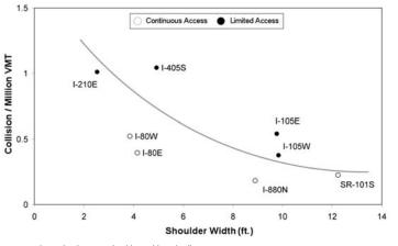
Figure 5 Relationship between shoulder width and collision rate.
