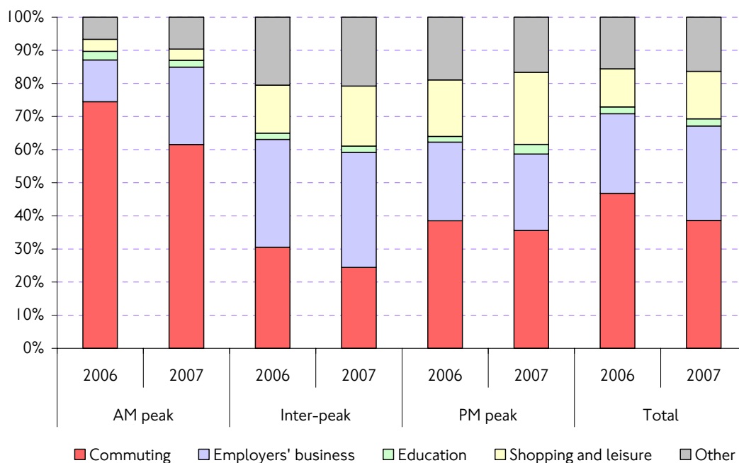
Figure 6.3 Purpose of trips crossing the six sites on the free passage route road side interview survey, all trips by private vehicles. 06:00-20:00, 2006 and 2007.
