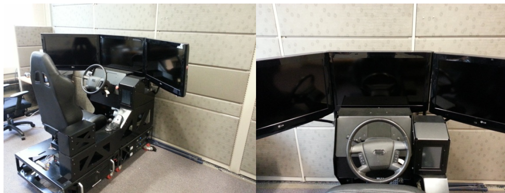
Figure 3.1. HumanFIRST portable driving environment simulator set up.
