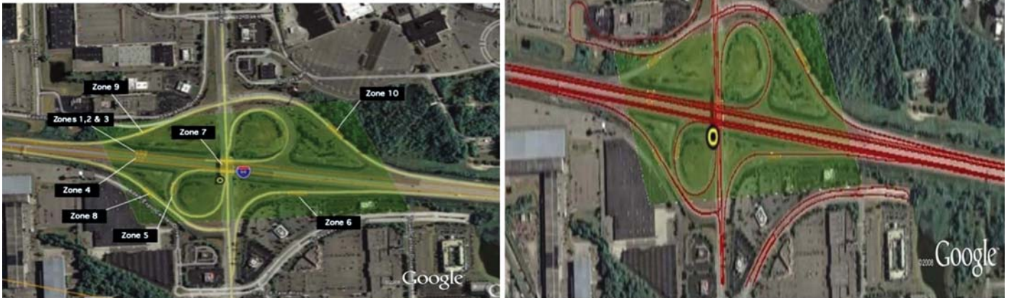
Figure 23. Tolling zones at the Michigan test bed (left) and cumulative vehicle passes (right).
