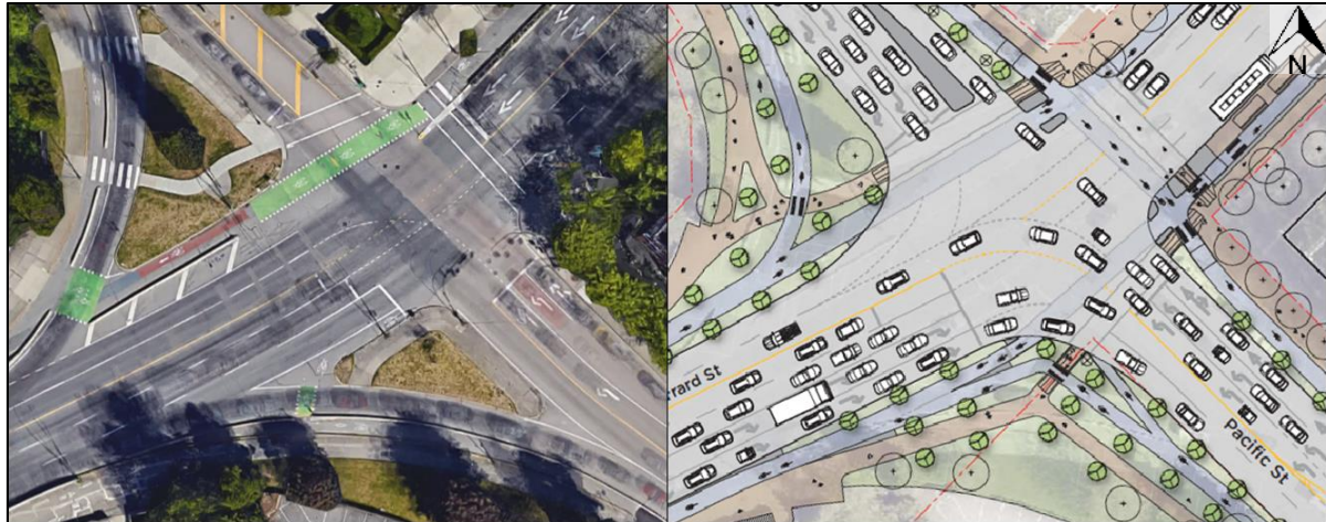
Figure 6: Current (left) and proposed (right) designs for the Burrard St. and Pacific St. intersection. Source: City of Vancouver [42].
